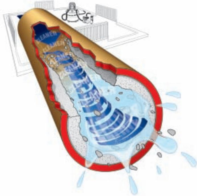
By connecting the powerflushing unit to the heating circuit in place of the system pump, boiler or radiator the system can be thoroughly cleaned of limescale and corrosion debris.
